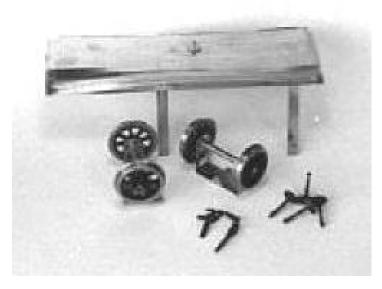
The roof has the inside planking etched in and these shew through on the top. There is a school of thought that maintains the roof planking was visible through the canvas. I have yet to see any pictures to support this view. However, I shall wait to see what it looks like when painted and, if necessary, add a layer of tissue "canvas" to hide it.
