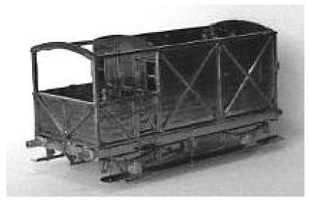
Solder cream and an RSU makes this job easy. The same pins were then used to help fix the spring to the axle guards and again, soldered from the rear. The top laminate is the one that is etched for the spring leaves. It has a nice long sprue on its convex face that holds it to the etch. Keep this intact so that when soldering up the
