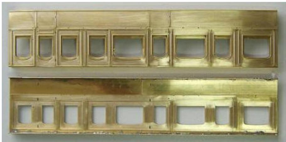
the curves are correct. The overlays can now be soldered in place as shown here.
