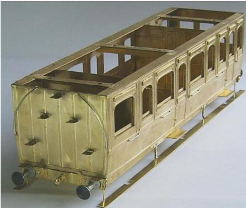
Here is the body virtually complete except for the outer door handles. The step boards need very careful handling and reinforcing with wire stays behind the fixing stanchions. There is also very little clearance for the Cleminson trucks so I would advise filing the cut-outs for the axle boxed a good deal deeper *before* fixing.
