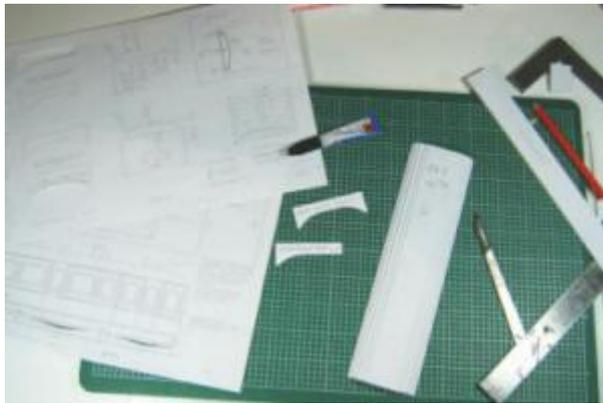
Cut out the profile pieces and set aside. Next, cut the sections of plasticard for the roof as mentioned in the instructions. It is difficult to measure the sections to the sizes in the instructions. They were originally worked out on a computer by Ivan. I found it difficult to cut sizes such as 55.51mm or 44.35mm and simply cut them to the nearest half millimetre over the size indicated.
