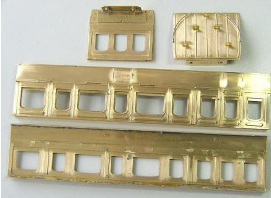
usual, I fitted as much as possible "in the flat". The only parts not fitted at this stage are the door handles. Ian and I are trying to source a lost wax handle to use.
