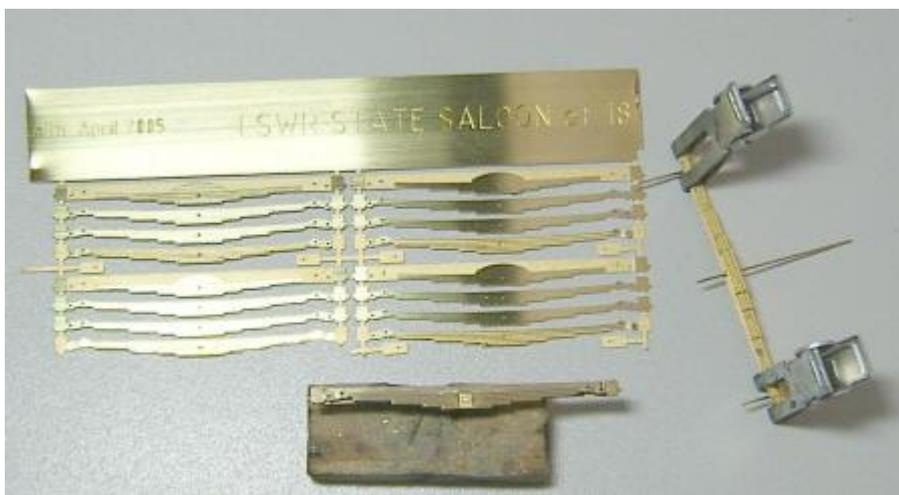
The kit arrived as an etched sheet about 550mm x 300mm bound in a couple of sheets of hardboard, together with comprehensive instructions, drawings, historical background, list of parts, a couple of bags of bits and castings and map of the etches.
