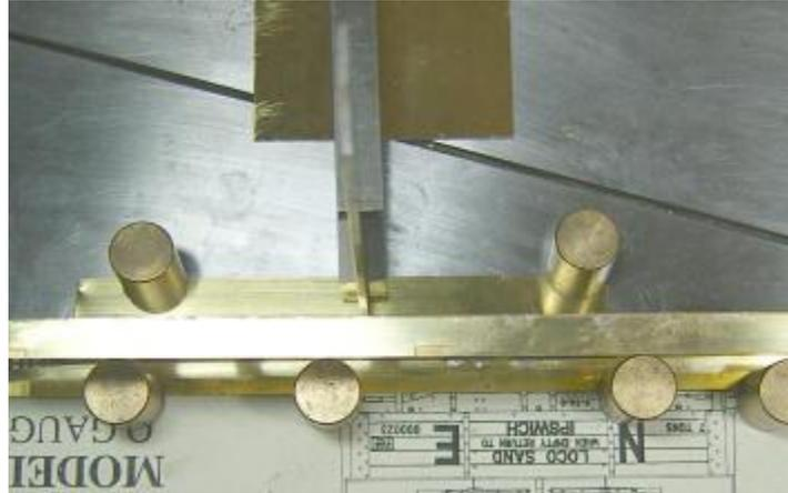
Here is the side with both rails firmly soldered in place with both the tumblehome and end curve in place. It was necessary to tweak them a little after soldering but
