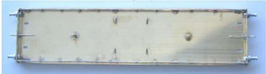
The coupling hooks are made from three layers of laminate that, once filed to shape, make up into excellent representations of the LSWR's version of the gedge hook. There are etched holes in the extension under the floor to take the buffer springs, most of which got cut off when fitting the Cleminson trucks to prevent fouling.
