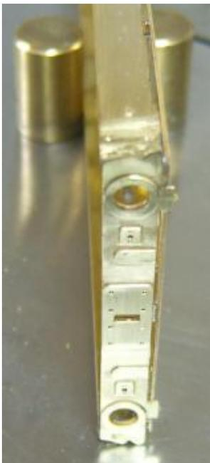
assembling the parts. Normal seaming is not an option here and so I soldered both the tabs in slots (4 each side and very accurate) and the spacing tabs. The floor itself also curves in at the ends. It is essential for this kit to file of the cusps for most joints. On occasion too it is necessary to open out the slots a little with a scalpel blade. All good signs of a well-designed kit in my view.
