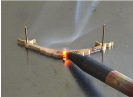
Heat is then applied with the probe. I would normally hold this down with a scalpel or similar as well but the other hand was operating the camera. The discolouration is normal and will disappear with normal cleaning ready for painting. The
