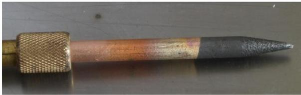
The flux from the solder cream does cause a build up of dirt that tends to reduce conductivity. Use a fibre glass brush to buff up the remaining copper to ensure good conductivity. The rod is pushed well down the holder and the brass ferrule forced down hard so that there is no wobble in the probe.
