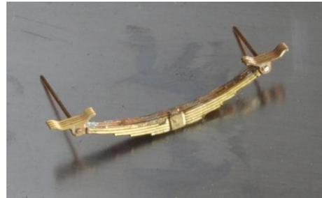
finished article, as you can see, needs no excess solder removing and can be fitted to the underframe immediately.
