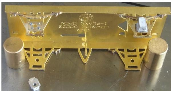
brass and a good helping of flux to the back of the casting.
