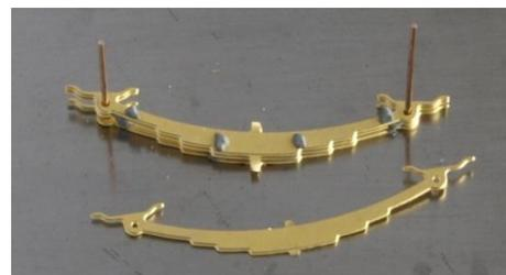
holes drilled in it to take lengths of 0.5mm wire at the spacing required for the spring.
