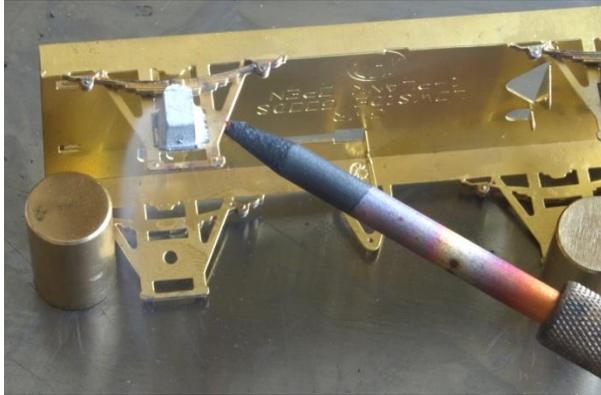
If it is not possible to apply the probe to the back, apply it to the side at the front, not to the casting itself. As soon as the solder flashes silver switch off the power. I generally blow on it as well to speed up cooling.
