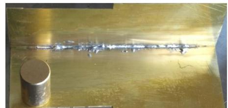
The solder cream has little gap filling capacity. To add a fillet use wire solder and run the probe along it and into the joint.
