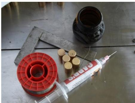
For this the job we will need an engineer's square, solder cream, magnets, wire solder and flux. The parts to be joined
