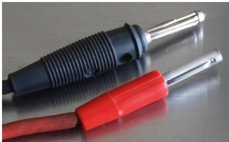
Cleanliness is important and it is critical that no power is lost in the chain from the unit to the work piece, so electrical joints must be tight. Here you can see that the plugs that go into the unit are cleaned to a bright shine. It is also important to keep the springs opened out to ensure that they fit in the sockets tightly.
