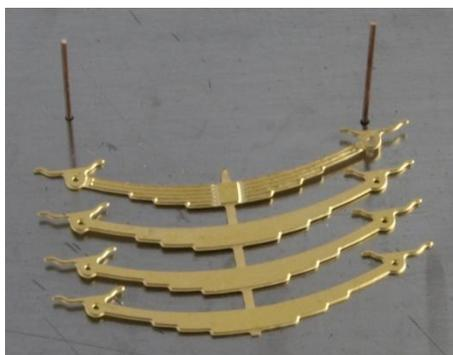
A tad more complex is joining laminated parts to make a component in this case a wagon spring. Wasting time applying, in this case, six layers of tinning is, for me, not an option. Here the steel plate has two
