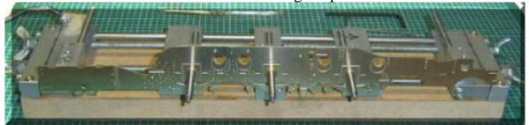
Add the next side frame with bearings and spacers and solder up the whole chassis (pictured below). Where one uses an RSU, clamp the negative terminal to the jig. You can see a substantial brass terminal I have bolted to the jig in the top left corner
