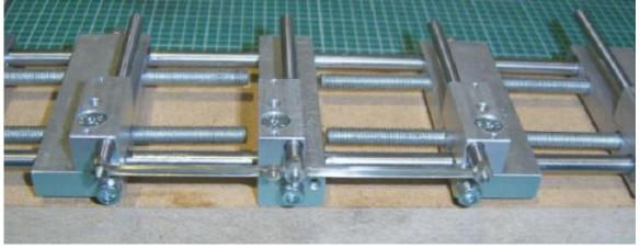
Now fit the side frame and solder the bearings in place.
