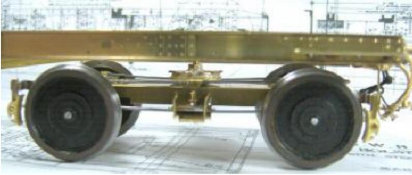
Bogies fitted to an underframe. The first without side frames fitted to shew how the parts go together and the two sets of piano wire springs. The second is ready for the body (to push the axles boxes down) and painting.
