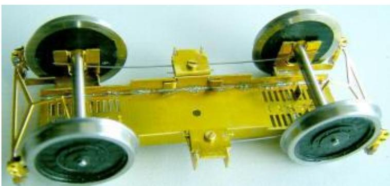
The same unit upside down with the wheels temporarily dropped in. The two bolt heads hold the clamping plate for the wheels springs. The instructions suggest 12BA but the holes are quite large and I found that 10BA was both easier to fit and less fiddly
