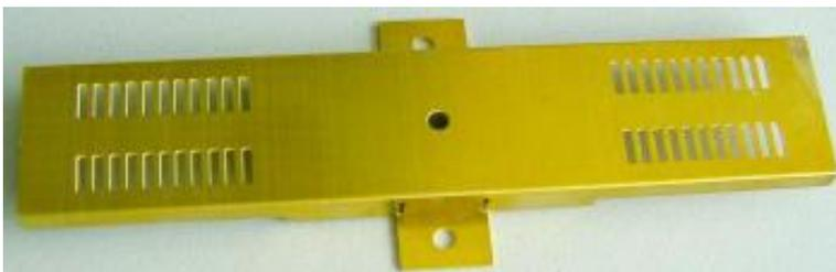
This fold-up base frame is the basis upon which the whole system works. The slots allow one to produce bogies with a wheel base between 6 to 11 foot centres in 6 inch increments.
