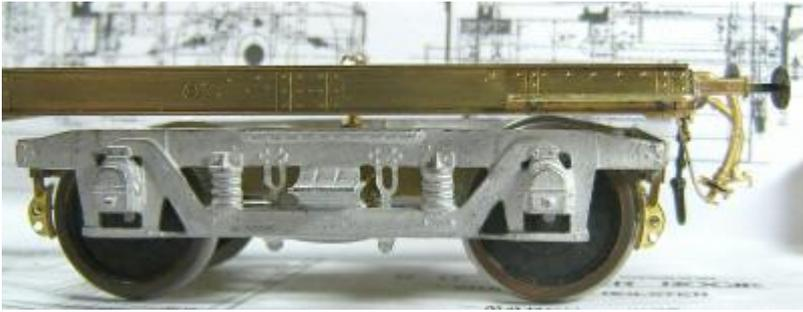
An excellent kit of parts that makes up into a robust unit that will support quite heavy weights (this carriage is in excess of 2lbs) depending upon what gauge of piano wire is used. It is not beyond
